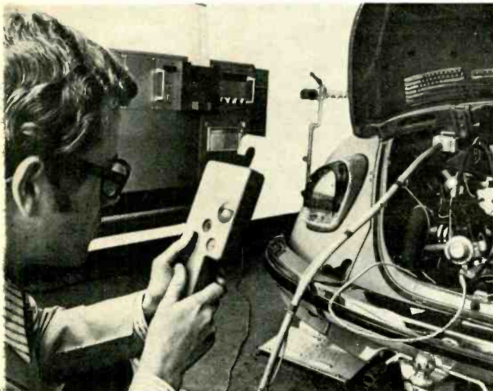
TECHNICIAN USES HAND-HELD INPUT UNIT to follow test countdown. Unit feeds the test findings into the computer at left.
