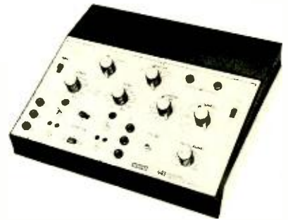
FIG. 6—EICO MODEL 443 is a typical solid-state semiconductor curve tracer.
