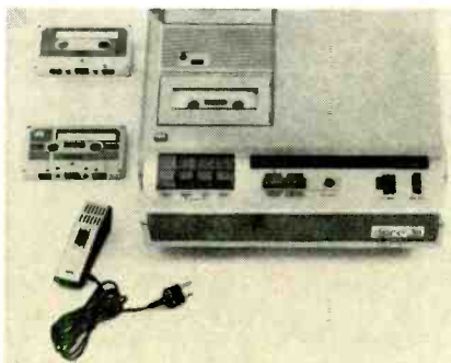
FIG. 1—AUTOMATIC TELEPHONE answering system; the Doro 311.
